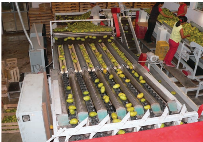
Automated fruit sizing on the packingline
