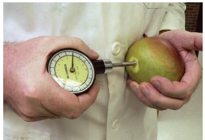
Measuring mango flesh firmness with a penetrometer
