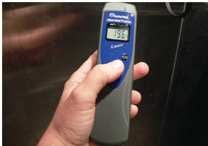
Measuring surface temperature with an infrared thermometer
