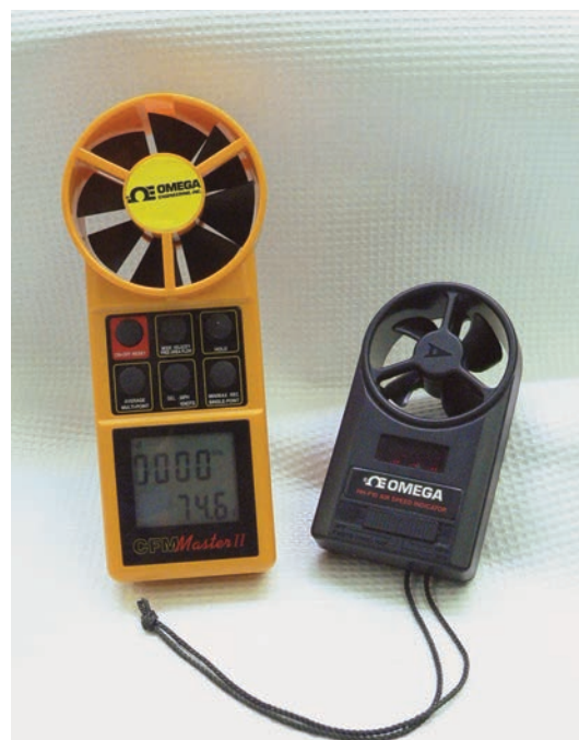
Vane anemometers used to measure air velocity
