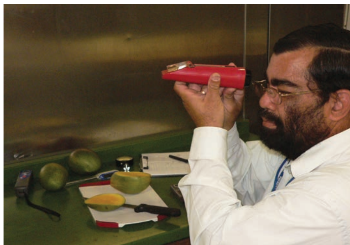
Measuring mango fruit TSS with a refractometer
