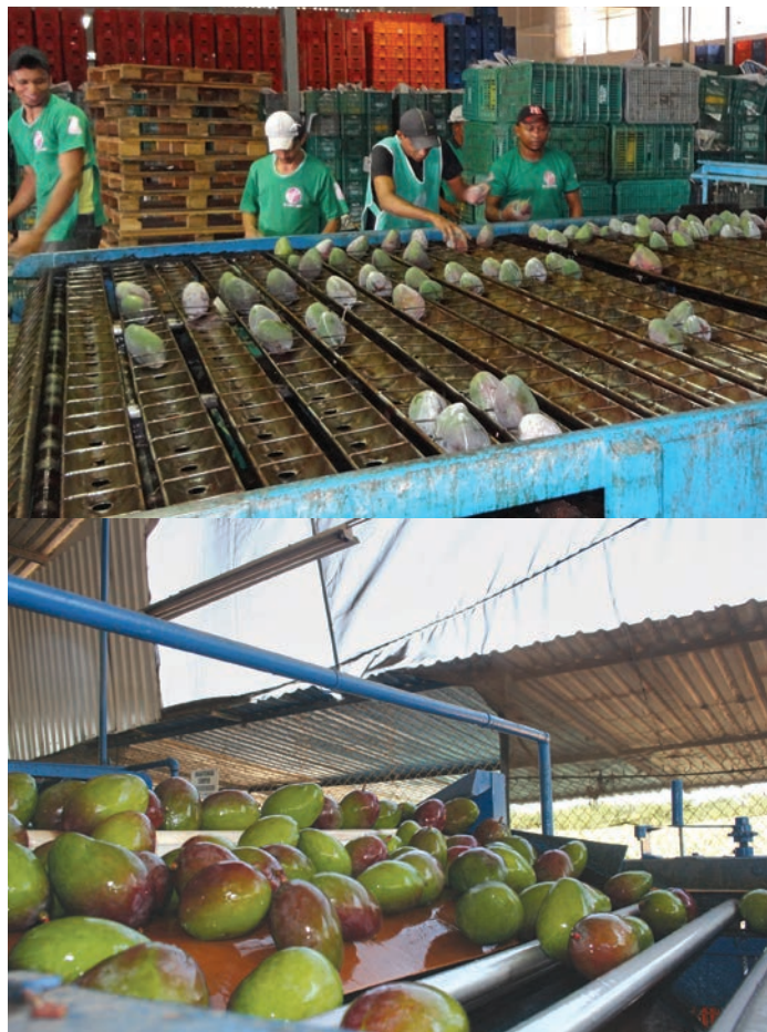
Initial fruit sizing by weight (top) and by dimension (bottom)
