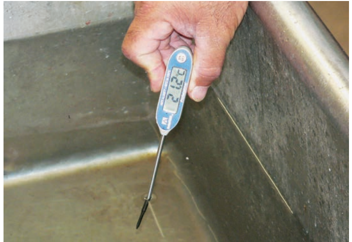
Measuring hydrocooler water temperature
