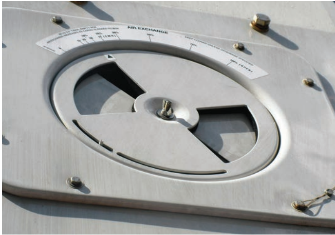
Fresh air exchange on a marine container
