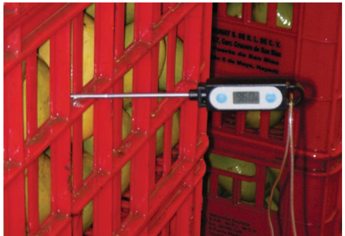
Measuring mango flesh temperature following hydrocooling
