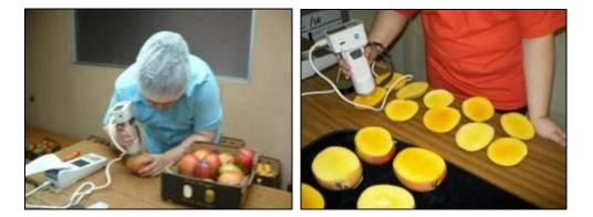
Pulp firmness was measured using a handheld manual penetrometer with an 8-mm Magness-Taylor probe. Measurements were taken on two sides of each mango and the average value of those measurements was reported as a pulp firmness for each fruit. Ten mangos were analyzed for each color category and/or variety after every storage interval.
