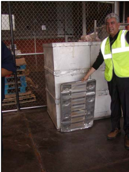
Pistons raise and lower the floor for easy loading
